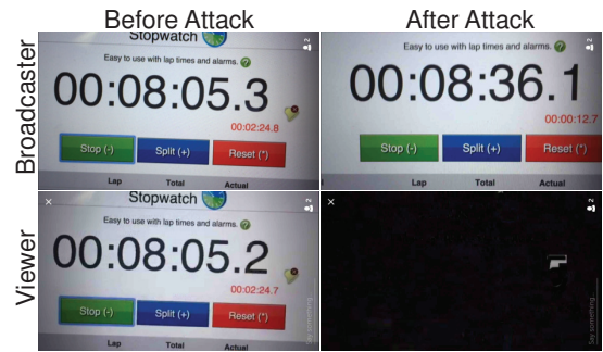
Figure 18: Screenshots of the broadcaster and viewer before and after the attack. After the attack, the viewer sees a black screen (tampered), while the broadcaster sees the original video.
